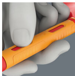
The recesses in the fast-rotating sleeve allow resistance to be generated by finger force. This allows the ratchet mechanism to be used even at low resistance of the screw.
